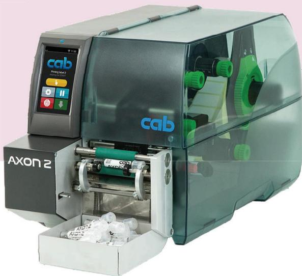
The Axon 2 is a low throughput volume tube and vial label applicator offering reduced operator involvement in comparison to manual labeling. The operator places the tube or vial in the applicator arms, taps the touchscreen icon and the labeled tube is either dropped into the tray or removed by hand.
