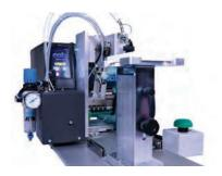
The S3200 precisely places labels on well plates for reduced waste and more efficient downstream processes. Semi-automated operation increases speed and productivity through reduced operator effort.
