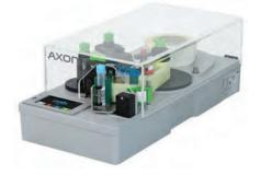
The Axon 1 was designed to print and apply labels quickly and efficiently to a range of tube and vial sizes. Capped or uncapped tubes or vials are placed vertically in the applicator arms, and with a tap of the touchscreen the tube is labeled.
