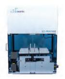
The Sci-print VX2 is a fully automated tube and vial labeler capable of handling a broad range of tube sizes. In addition to print and apply automation, the Sci-print VX2 can be configured to sort racked tubes, receive bulk tubes, uncap/recap, fill and/or scan barcodes.
